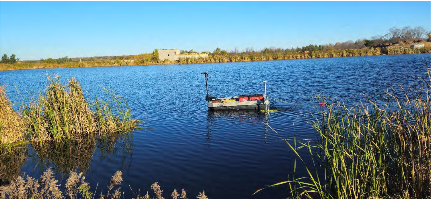
Digital Image 2. Wiarion Biosolids Aerated Cell #3 (North). Remotely Controlled Hydrographic Survey Vessel.
