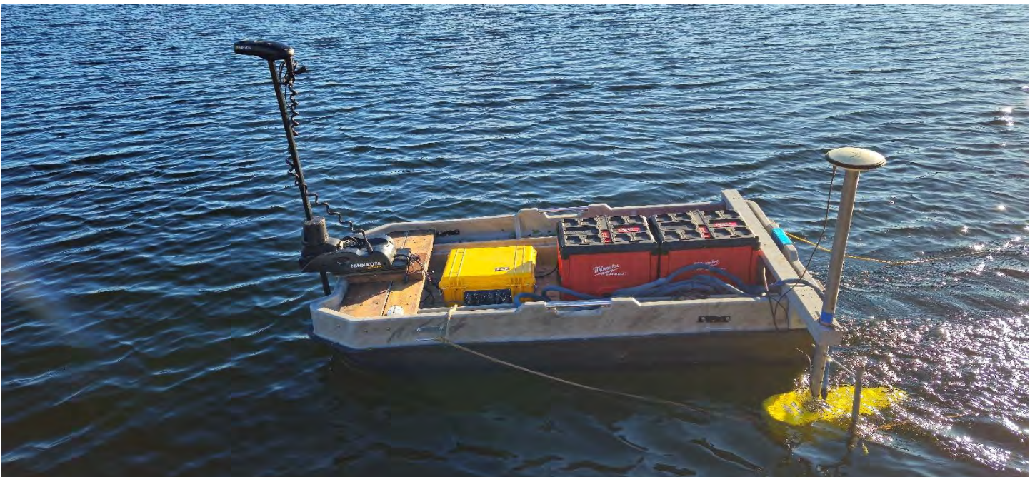
Digital Image 3. Wiarion Biosolids Aerated Cell #3 (North). Remotely Controlled Hydrographic Survey Vessel.
