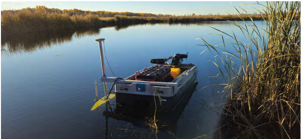
Image. OCWA – Warton Biosolids Aerated Cell 3. Unmanned Remote Controlled Hydrographic Survey Vessel.
