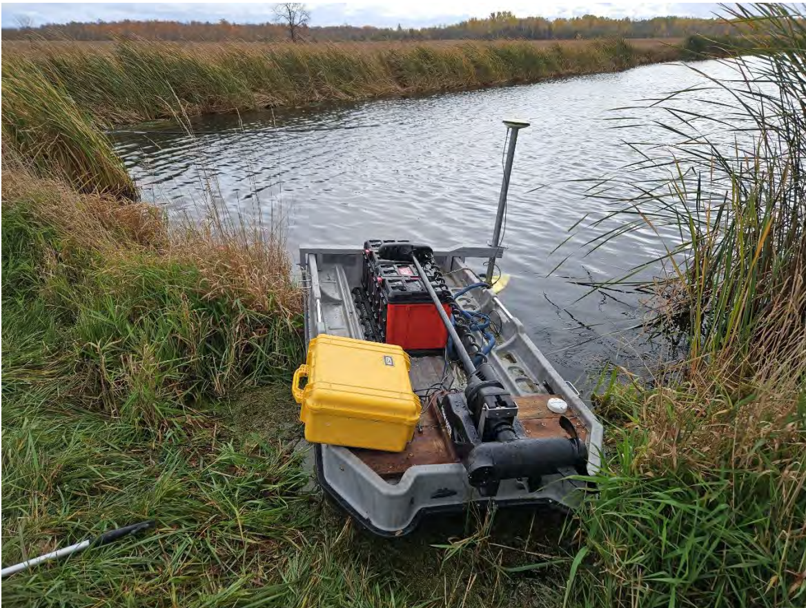
Digital Image 1. Warton Biosolids Aerated Cell #2 (Middle). Remotely Controlled Hydrographic Survey Vessel.
