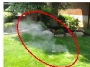
The “smoke” being used is a non-toxic coloured vapour that has no harmful effects on people or pets and is non-staining. The test involves forcing this “smoke vapour” into the sewer system to replicate water flow and to identify entry and exit points for water. The smoke will dissipate quickly shortly after the test is completed.
